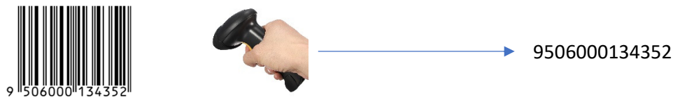
Figure 1 The basic message when a 1D barcode is scanned – just the digits
